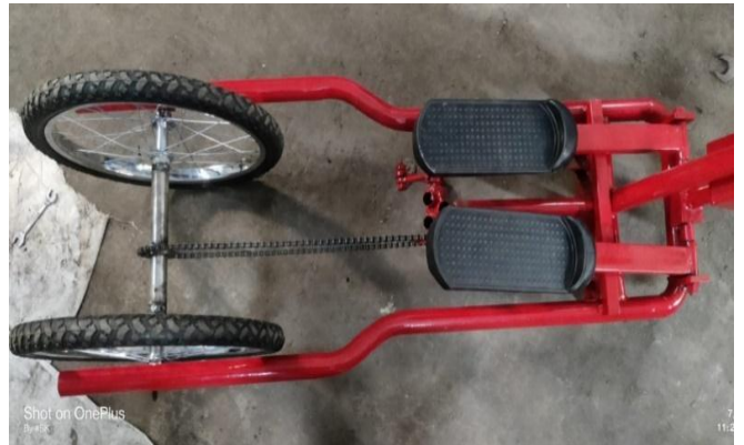
Fig -: 9 Assembly of stepper and wheels to chassis
