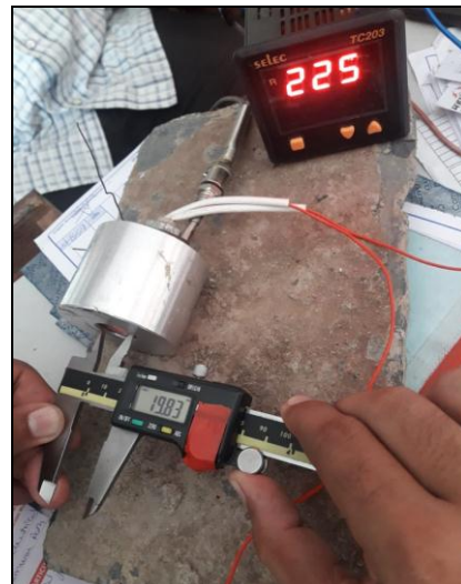
Figure 5. Thermal Expansion of aluminium rotor bore
