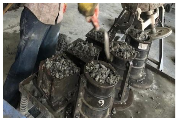
Fig - 3: Casting of Specimens
