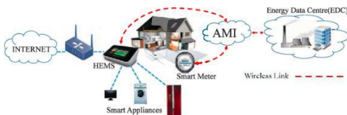
Fig.7. Smart Metering System with 5G network
