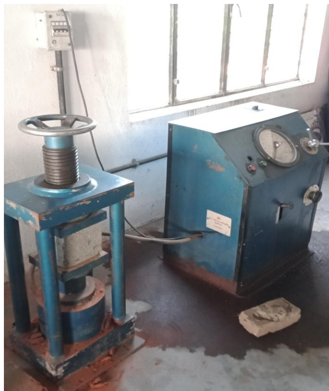
Figure 5: Compressive strength test
