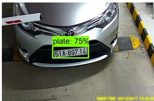
Fig-13: Examples of the detection of tiny and skew LPs using the SSD network
