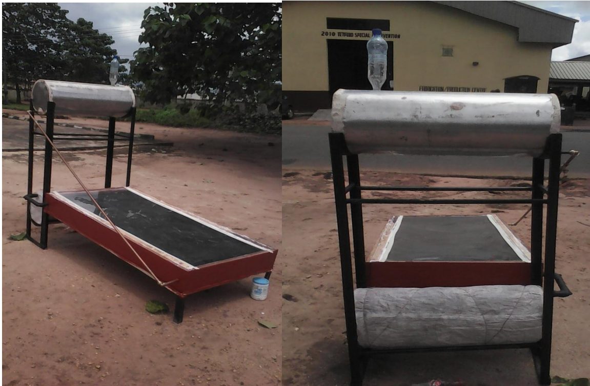
Fig. 2 side and back view of the serpentine solar water heater.
