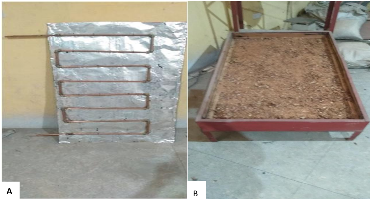
Figure 1 (a) serpentine copper tube (b) wood chips used as insulator material
