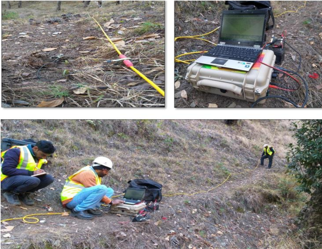
Figure 3: Instrument used for the 2D resistivity test
