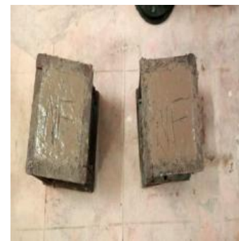
Fig -11: Casting of ferrock cement concrete
