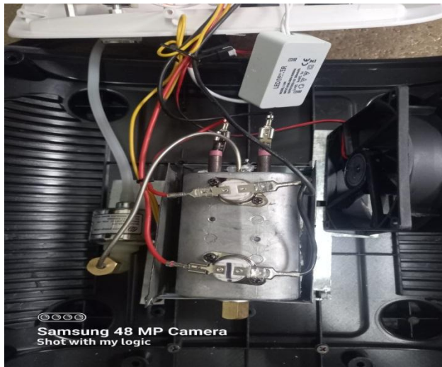
Fig 4: Heater of Fogging Machine
