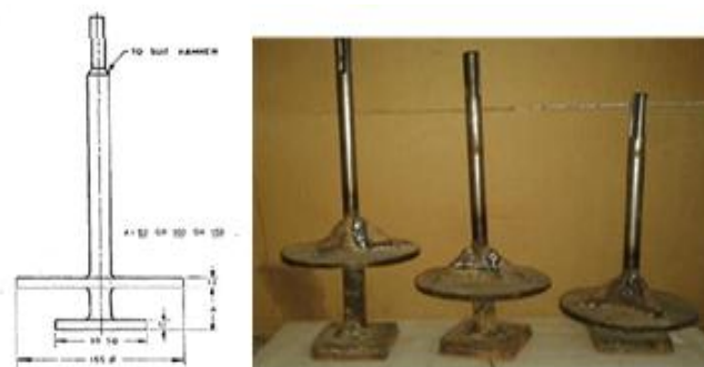
Figure 5. Tampers for use with a vibration hammer for unconfined Compressive Strength Test [(IS 4332 (Part V) - 1970)]
