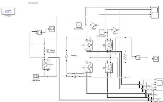
Fig -5: Simulink model of Modified MLI
