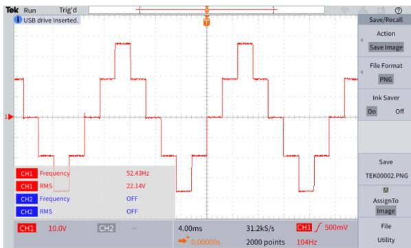
**Fig -15:** Output Voltage from Breadboard connection
