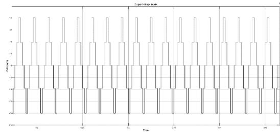
Fig -7: Output Voltage of modified MLI
