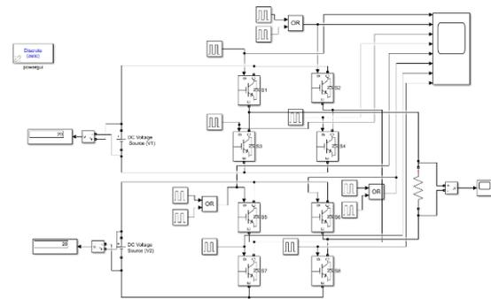
**Fig -2:** Simulink model of CHBMLI
