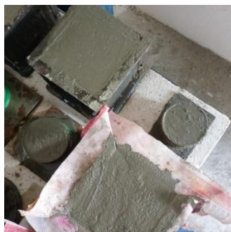
Fig. 7 casting of specimens with CPF liner
