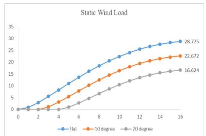
Chart -38: Variation of displacement for static wind load
