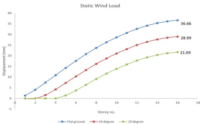
Chart -34: Variation of displacement for static wind load
