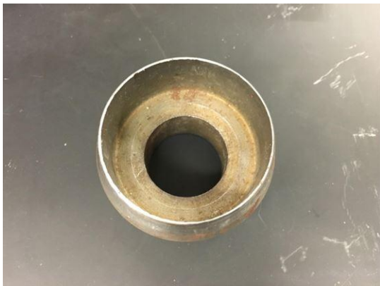
Figure: Die tool for creating acoustical sample
