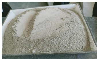
Fig-3: 43 Grade OPC Cement
