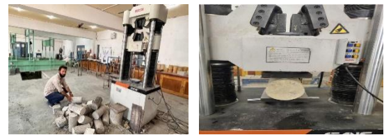
Fig.-10: Split Tensile Strength Test
