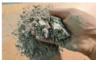
Fig.-1: Washed Bottom Ash
