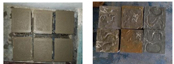
Fig-5: Casting of Cube
