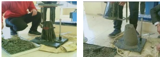
Fig.-7: Slump Test
