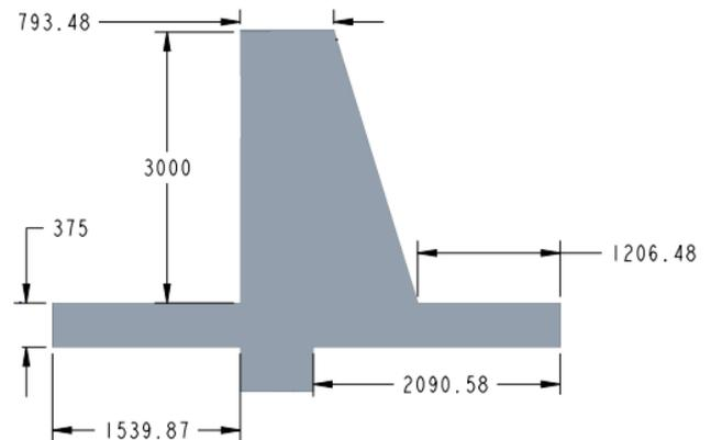
Fig -1: Model of Normal Retaining wall with Dimensions in mm
