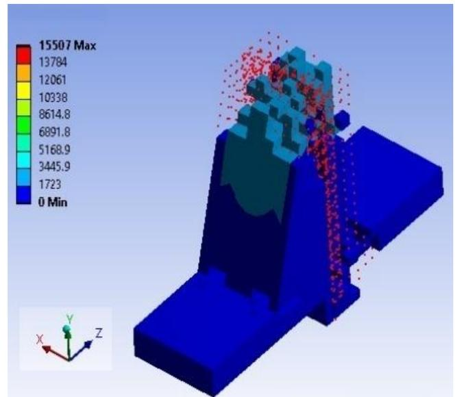
Fig -5: Deformation diagram of Normal Retaining wall under 1500kg TNT blast
