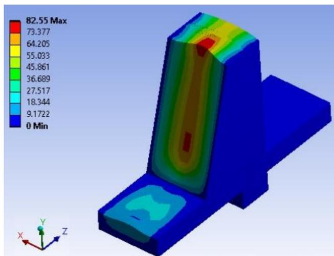
Fig -3: Deformation diagram of Normal Retaining wall under 1kg TNT blast
