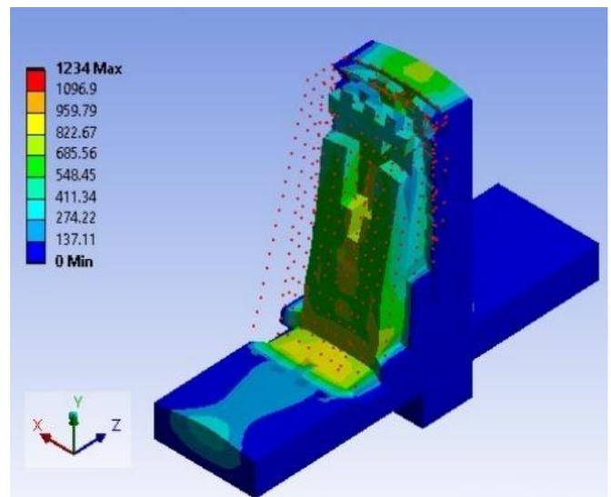
Fig -6: Deformation diagram of Sandwich Retaining wall under 1500kg TNT blast
