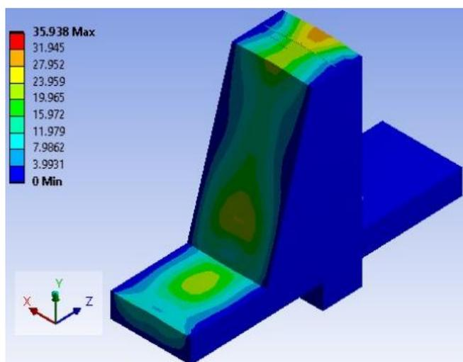
Fig -4: Deformation diagram of sandwich Retaining wall under 1kg TNT blast
