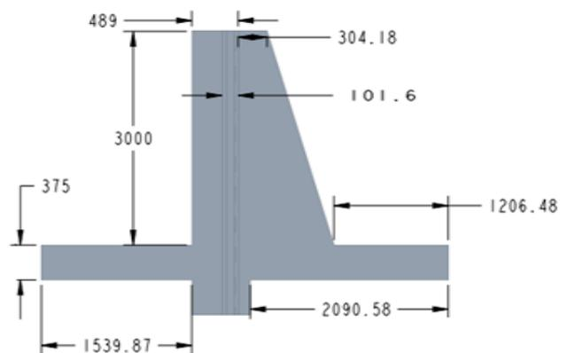
Fig -2: Model of Normal Retaining wall with Dimensions in mm
