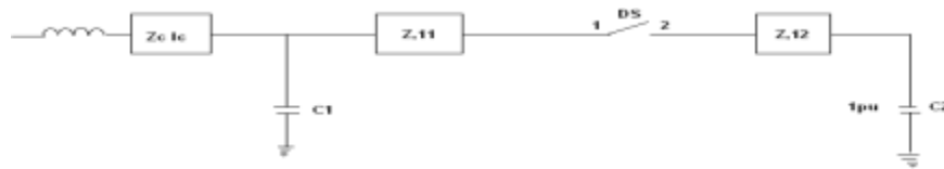
Fig 1. Equivalent circuit of GIS
