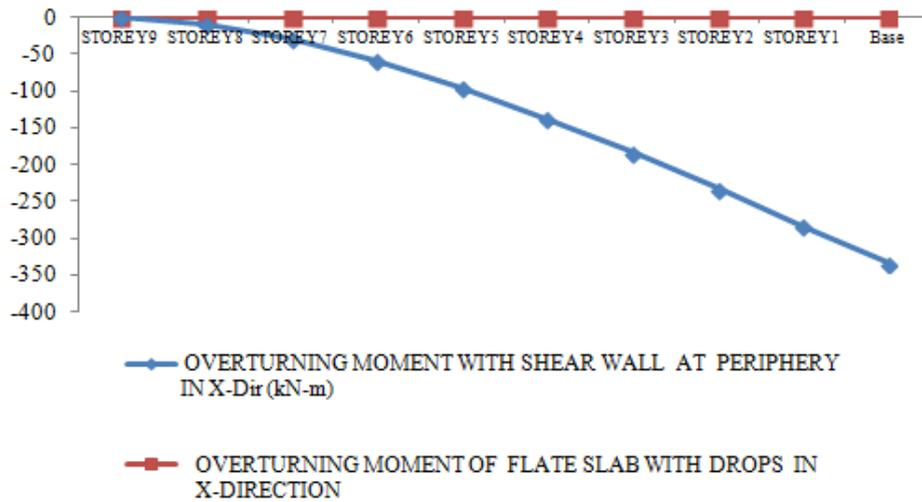
The restraining moment for building with shear wall at periphery is more as compared to building for flat slab with drops. According to IS 456:20000, Cl. 20.1, structure stability in the event of resisting moment must be larger than 6/5 times the maximum moment due to the normal dead load and greater than 7/5 times the typical applied loads.
