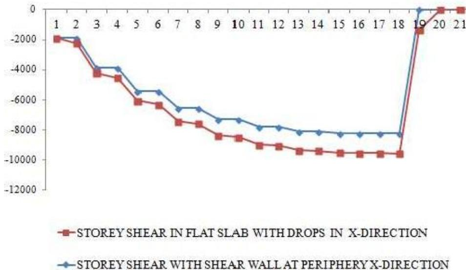
The storey shear in x direction with shear wall at periphery has more resistance to storey shear than flat slab with drop. Thus; the building is much stable under lateral seismic loading with periphery respect to flat slab with drop.
