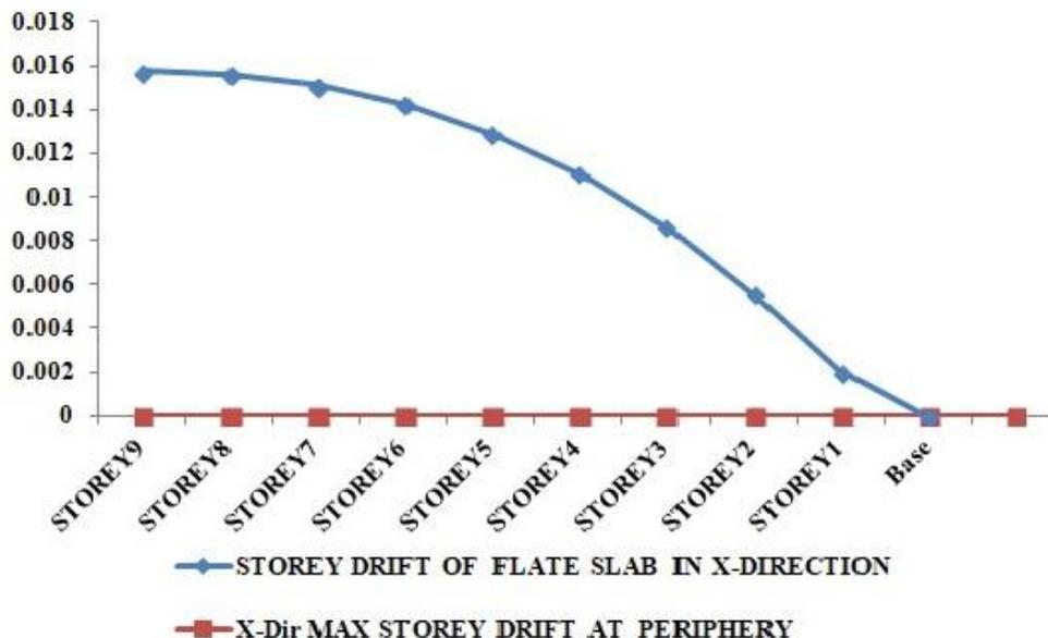
According to the following charts, the storey displacement and drift will be less at the bottom and higher at the top. The average storey displacement of flat slab as per IS 456:2000, Cl. 20.5, shall not exceed H/500 for lateral sway at top, where H is the building's entire height. According to IS 1893(Part -I) Cl. 7. 11.1, the minimum storey drift shall not be greater than 0.004 times the storey height.
