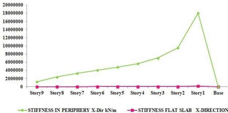
The stiffness of model with shear wall at Flat slab shows lower stability as compared to model with at periphery. Thus At periphery provides more stability to building under lateral loads.
