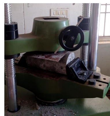
Fig-5: Split Tensile Strength Test
