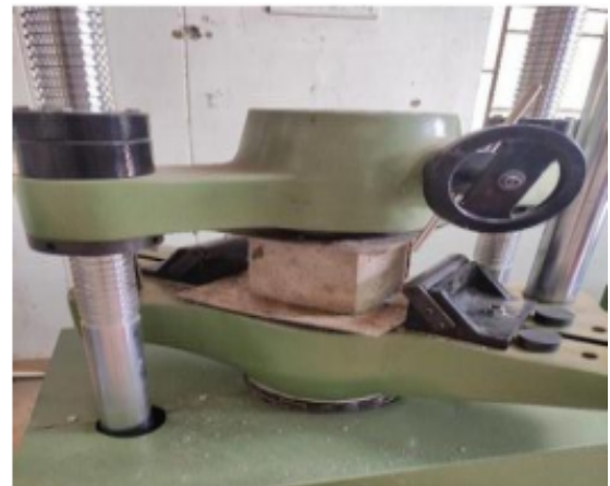
FIG-5: Compressive strength test on concrete
