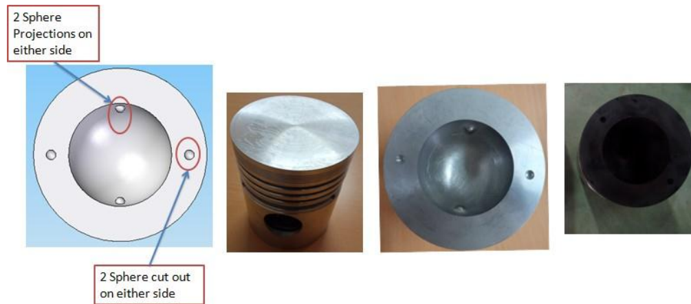
Fig.1- Modified piston of 2 cutouts and 2 protrusions on piston and piston bowl
