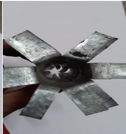
Fig-3: Top view of the swirl enhancer
