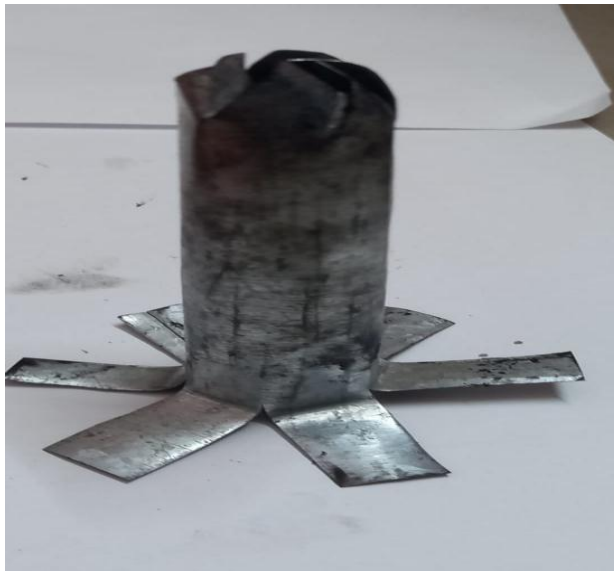
Fig-2: Side view of the swirl enhancer
