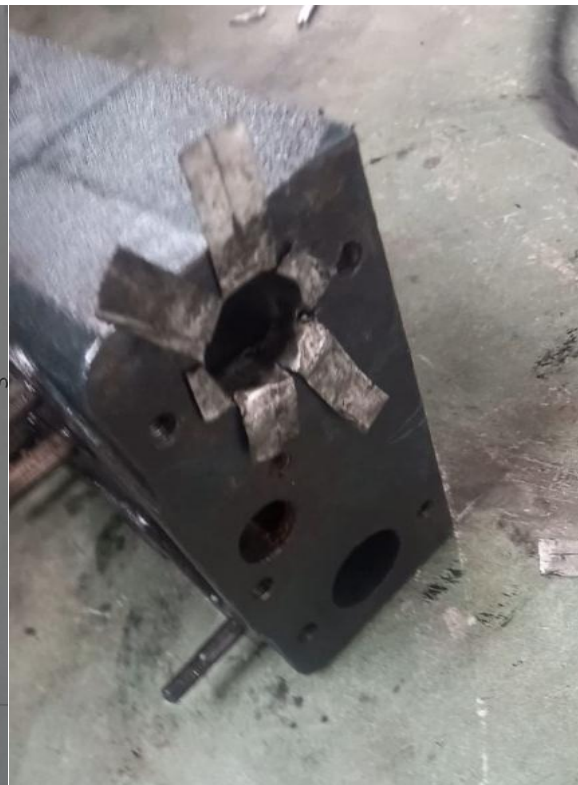
Fig-5: Swirl enhancer inserted in a cylinder head
