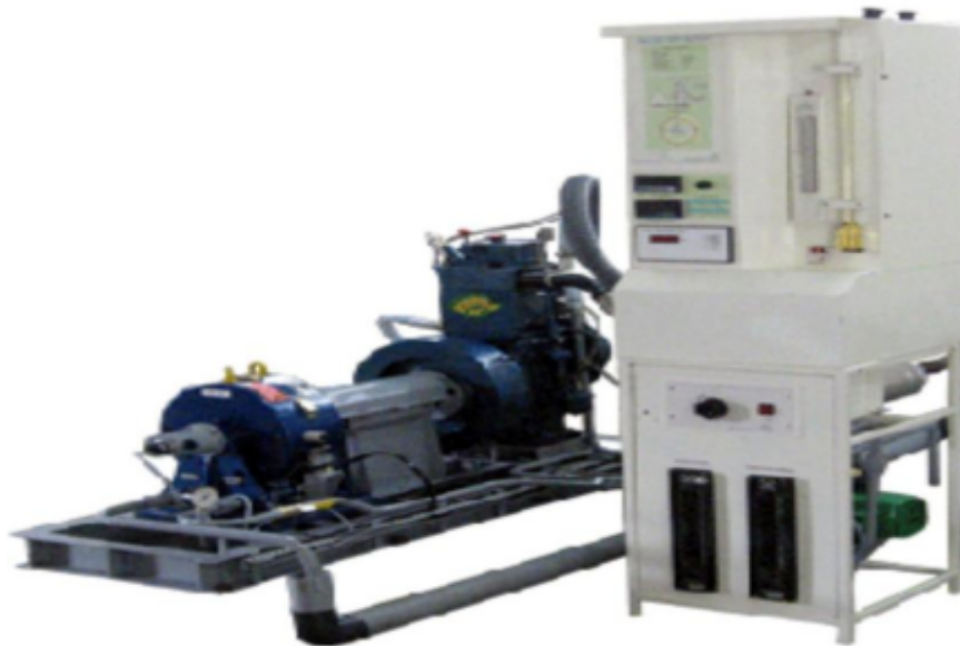
Fig-8: Computerised diesel engine test rig
