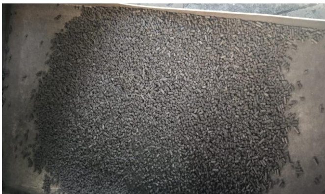
Fig -2 4x 30 size, impregnated coconut shell activated carbon.
