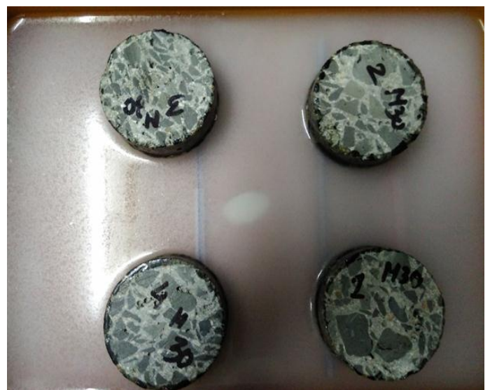
Fig -2: Sample Preparation for Sorptivity Test
