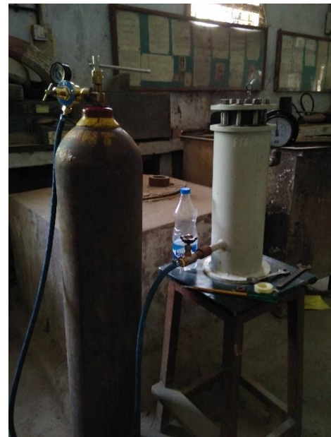
Fig -1: Test set up for Oxygen Permeability
