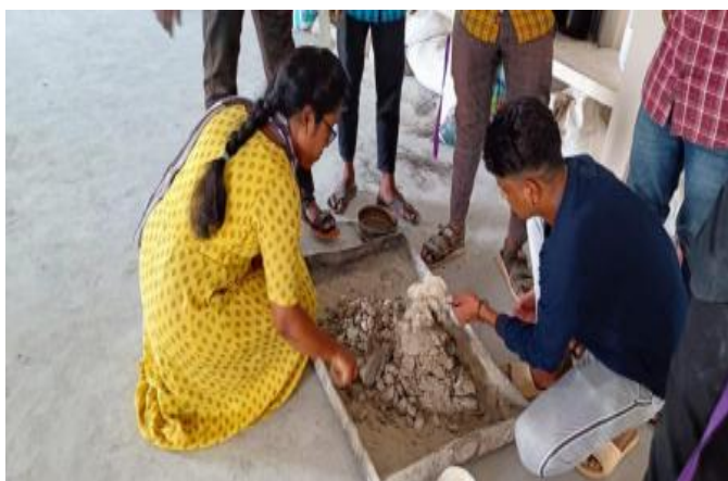
Fig No 3.3: Preparing paste for Brick molds
