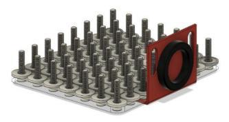
The tray used upcycled acrylic sheets from the window pane. Acrylic was drilled as per the design. A right-angle bracket from the headstock assembly of the CNC was used to hold the acrylic and the magnet together. We used an off the shelf magnet with the carrying capacity of approximately 2 kgs.
