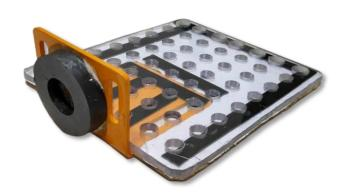
This tray created the following improvements: The workers now did not have to remember the number and sizes of bolts for the assembly, as when they arranged the tray with the bolts it is made sure that they have just the required bolts. The magnetic support of the tray made it very versatile as it can be attached on any section of the sheet metal assembly. Due to which there was a reduction in the worker's hand and feet movement.
