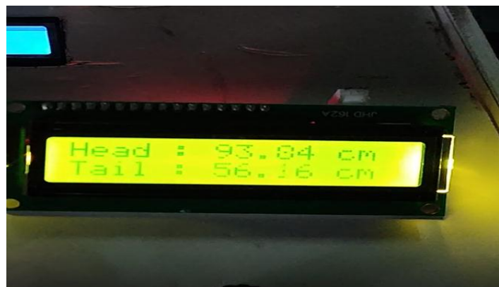
Fig -16: Distance between head and tailstock
