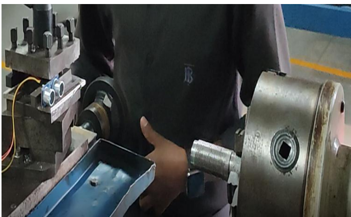
Fig -20: Ultrasonic sensor placed on toolpost
