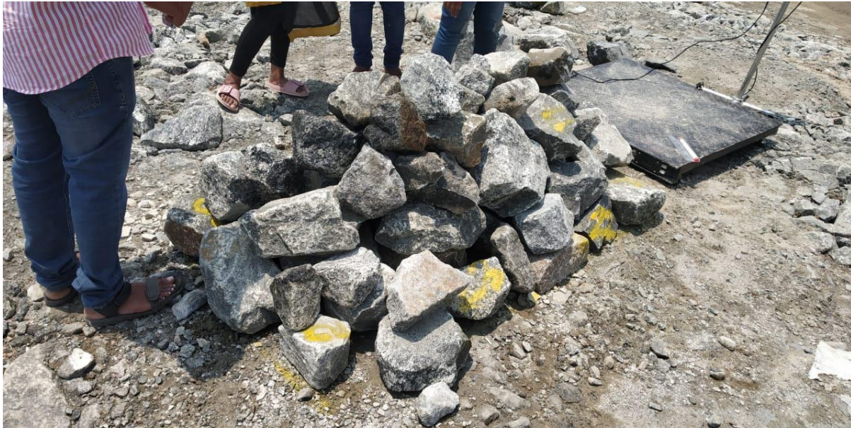
FIG3 MINIATURE EMBAKMENT USING CUBICAL STONES
