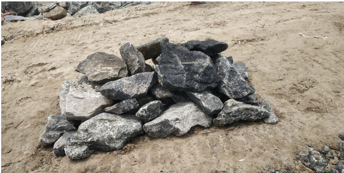
FIG 6 MINIATURE EMBAKMENT USING FLAKEY STONE
