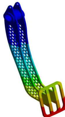
Maximum displacement = 2.6mm
