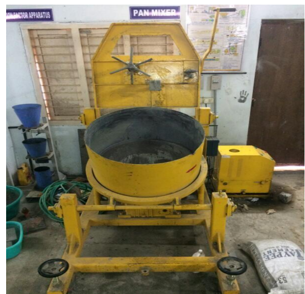
Fig-1: Pan mixer used for mixing
