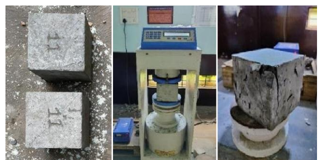
Fig-4: Compressive Strength Test of Cubes
