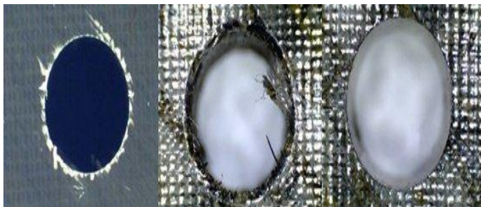
Fig -4: Glass fiber, jute fiber and hybrid Drilled hole
