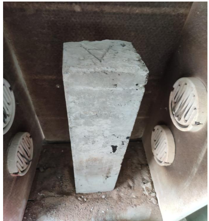
Fig 1: Heating of Beam at 500°C
