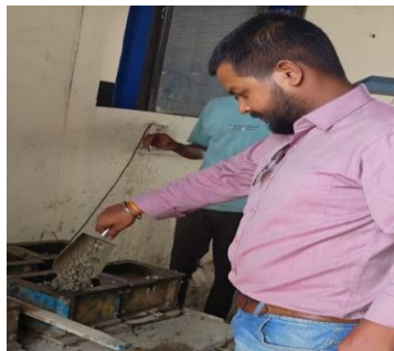
Figure-2 Cube Casting
