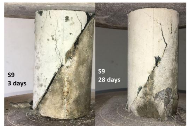
Fig.10 .Slant shear test specimens with cracks in GPC and PCC region [38]
