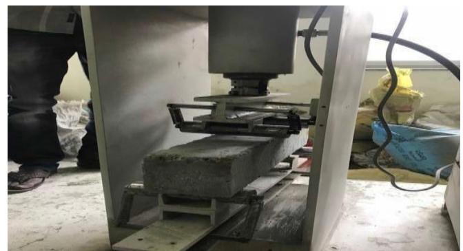
Fig -4: Flexure Test for specimen
