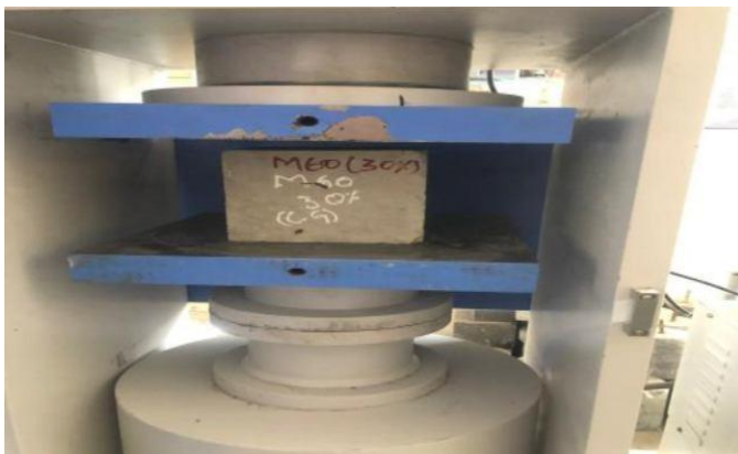
Fig -2: Specimen test in compression
