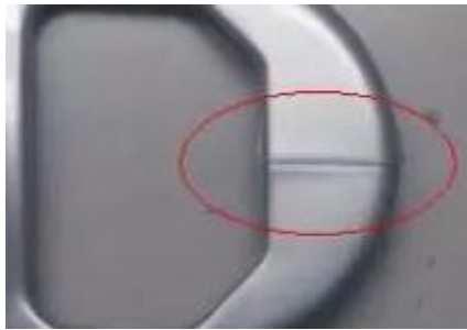
Fig -2: Weld line
