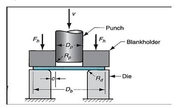
In general, the process of shearing and punching include opposition of forces that are applied to a material leading to tool penetration and workpieces fractures combining. The characteristics of the material and the figure of a tool influence the outgrowth anticipated on the processes . Different shapes can be generated ranging from introductory shapes like the indirect part on the far right in Figure 4 to more complex shapes similar as the one on the left wing.
