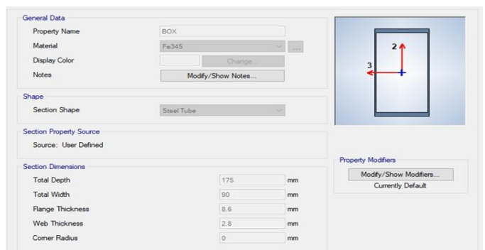
FIG-2: Section dimensions of 175 mm Box-Section The following table gives the analysis results.
