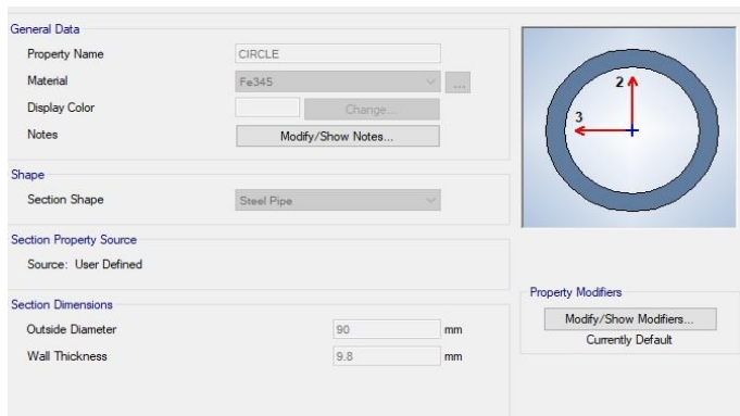
FIG-3: Section properties of circular section
