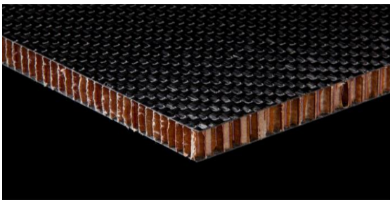
Fig -2: A honeycomb carbon fibre sandwich panel
