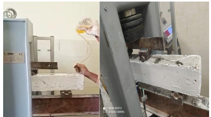
Fig -3: Test Sample during and after Injection
