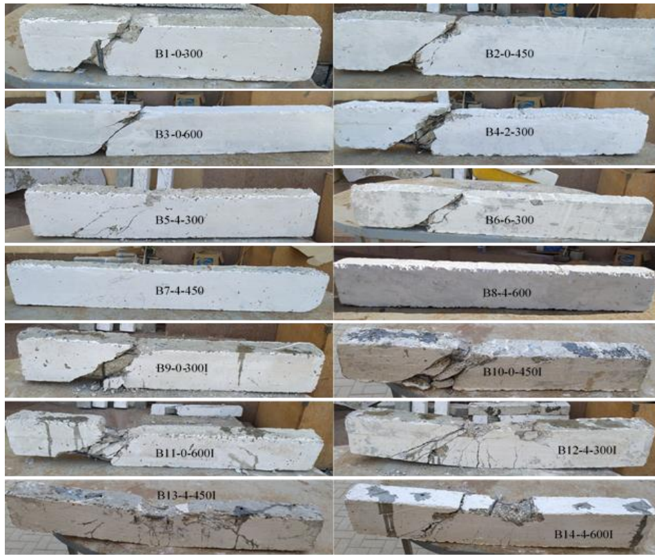
Fig -5: Cracking of the tested beams
