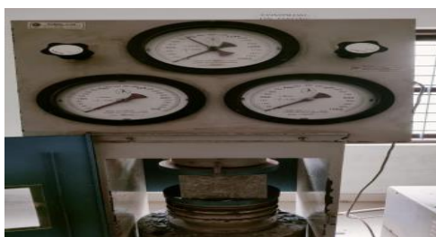
Figure 3: Compressive testing machine
