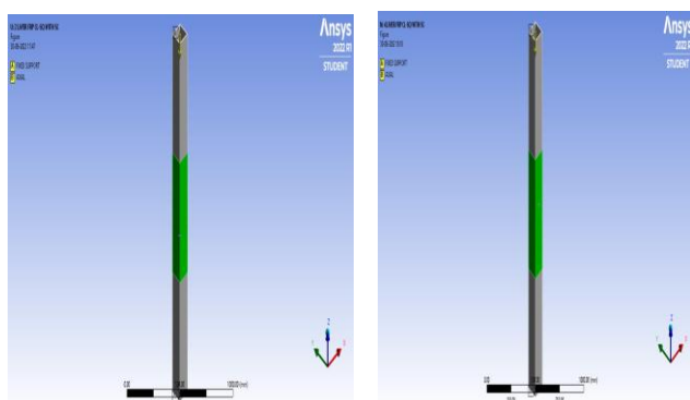
Fig-33: Boundary condition of SHS wrapped in 2 and 4 layers of hybrid FRP under compression loading
