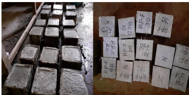
Fig-4: Concrete casted in mould and de-moulded cubes
