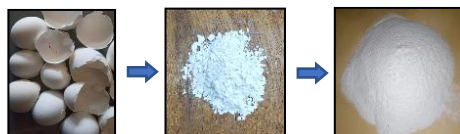
Fig 2: Egg shells to flakes and then into powder (left to right)
