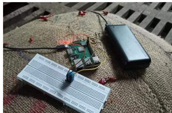
Fig 2. (Right) Raspberry Pie based IoT setup used to record temperatur
