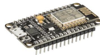
Fig-3: IOT Esp8266 Node MCU
