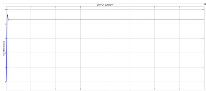
Fig-4: Output current waveform of open loop DC-DC SEPIC converter
