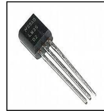
Fig 5 LM35 Temperature Sensor
